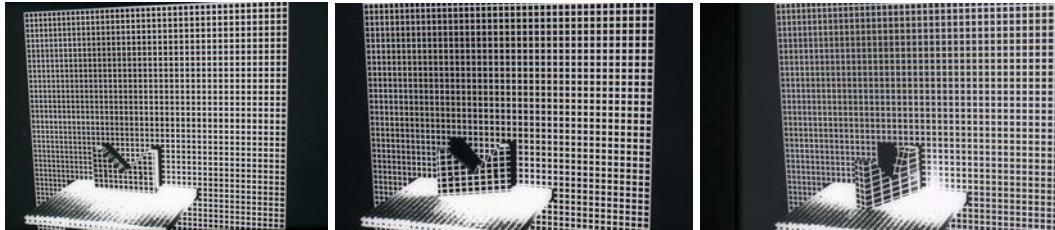
Documentation of a 3D object against reference plane illuminated with structured light, 1984
